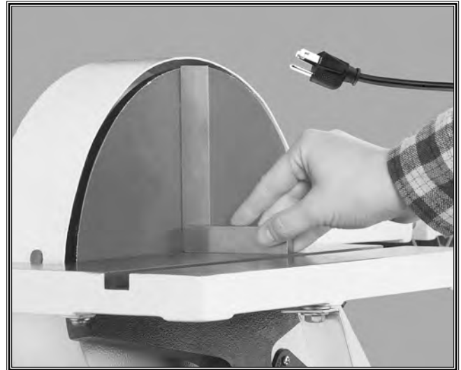
Figure 29. Checking table alignment.
