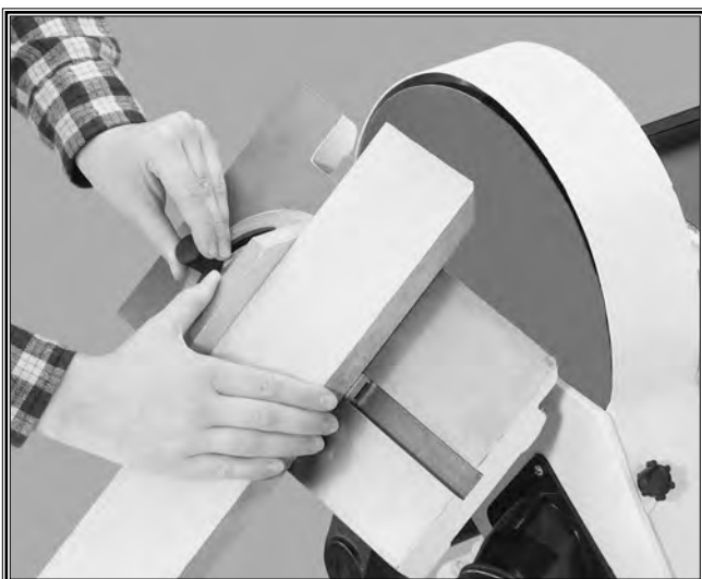
Figure 37. Using table to sand angles.
