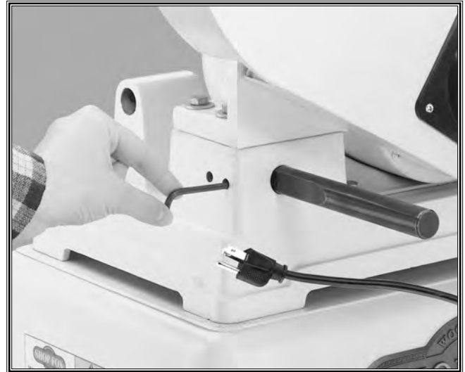
Figure 15. Tightening the setscrews.
