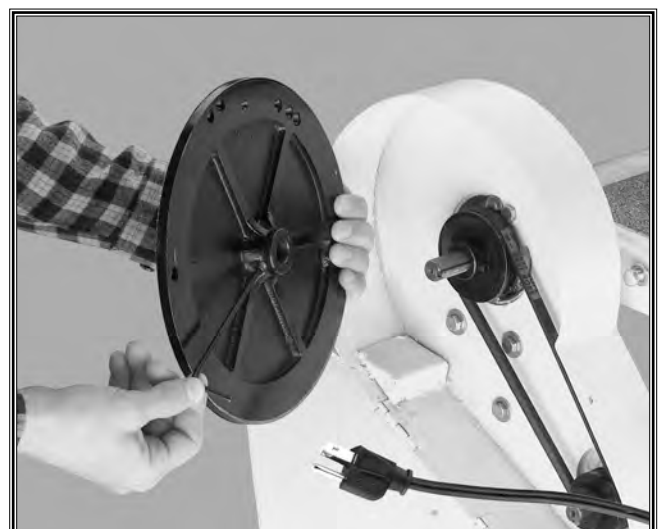
Figure 11. Installing sanding disk.
