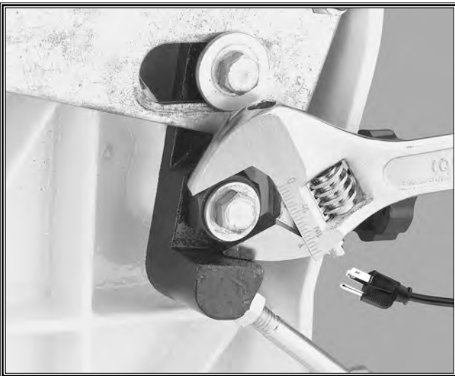
Figure 21. Loosening eccentric bolt head. (Belt Removed For Clarity)
