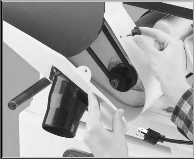
Figure 26. Opening pulley door.
