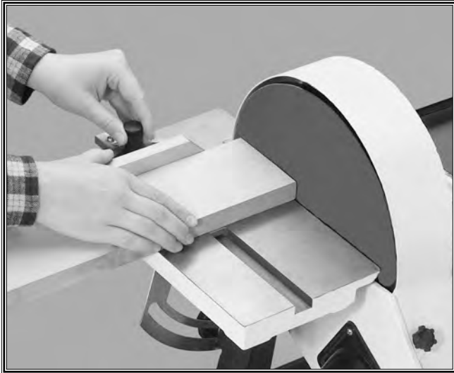
Figure 35. Sanding end grain.
