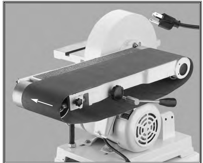
Figure 18. Installing the sanding belt.
