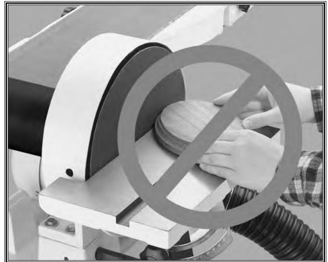
Figure 4. Never use the right side of disk. Upward rotation of disk can propel workpiece into the air.
