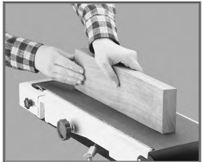
Figure 33. Sanding without back stop.
